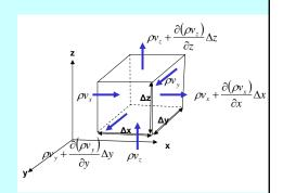
$$K \left[ \frac{\partial^2 h}{\partial x^2} + \frac{\partial^2 h}{\partial y^2} + \frac{\partial^2 h}{\partial z^2} \right] = S_s \frac{\partial h}{\partial t}$$
