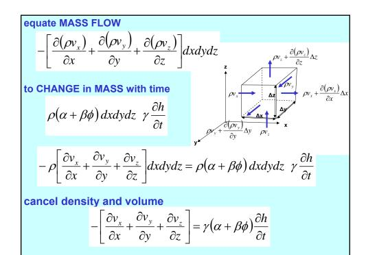
$$-\left[\frac{\partial v_x}{\partial x} + \frac{\partial v_y}{\partial y} + \frac{\partial v_z}{\partial z}\right] = \gamma (\alpha + \beta \phi) \frac{\partial h}{\partial t}$$
