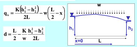
$$h_{\text{tream}} = \sqrt{h_1^2 - \frac{\left(h_1^2 - h_2^2\right)d}{L} + \frac{w}{K}(L - d)d}$$
