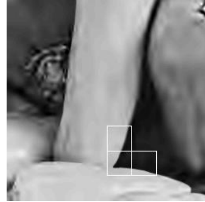
Fig. 4. Portion of Peppers image coded using W-SFQ optimization. Rate = 0.07 bpp, PSNR = 29.25 dB. The three boxes highlight some of the blocks described by curve trees.
