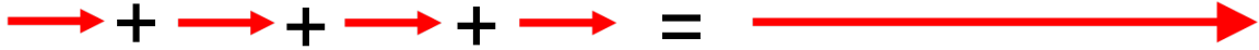
Figure 3.15. An illustration of the synthetic aperture concept: a large synthetic source can be constructed by adding small sources.
