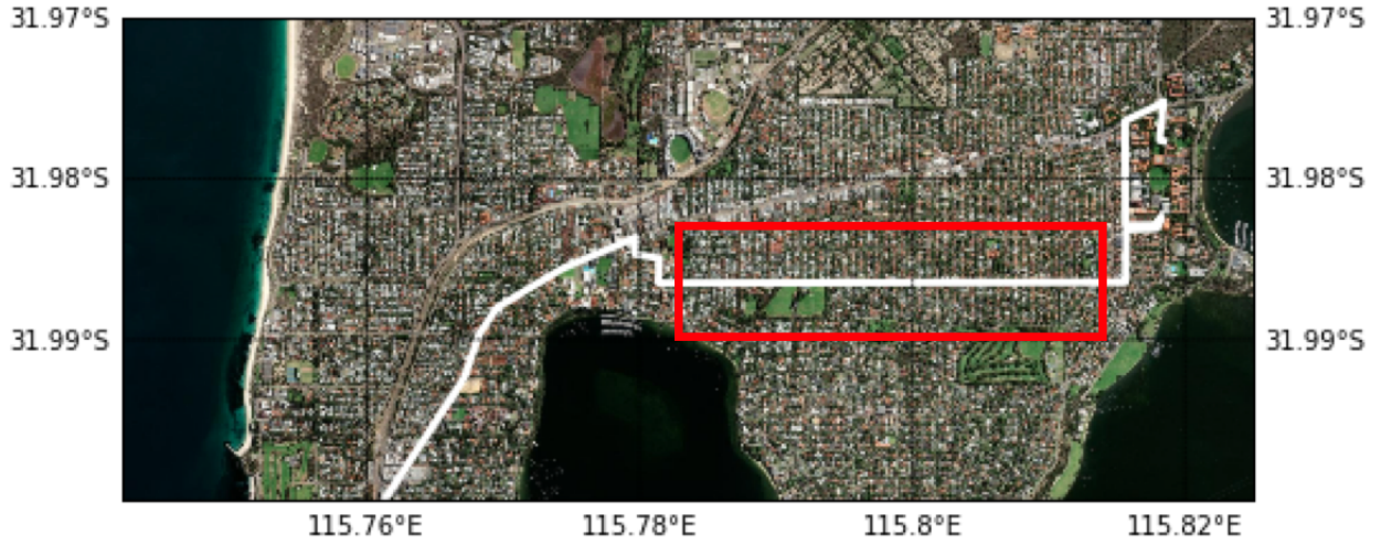
Figure 4.1 Map of the Western Suburbs of Perth, Australia with a deployed DAS fiber (white line). The red box indicates the 4 km linear section of the DAS fiber that is used for seismic interferometry and our wavefield reconstruction example. Modified from Figure 1 in Shragge et al. (2021).
