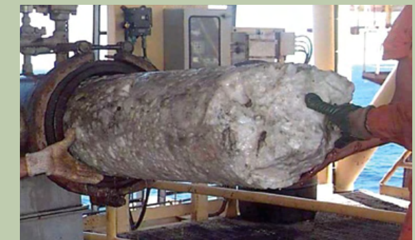
A hydrate plug. Courtesy of Petrobras
