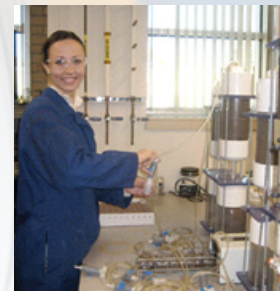
Tara Davis performs several leaching column tests for gold ores.
