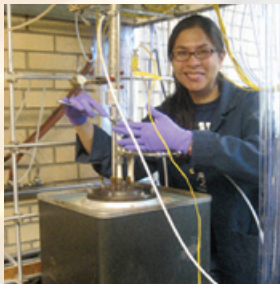
Judith Gómez works on a new electrolysis deposition method to produce high purity boron.
