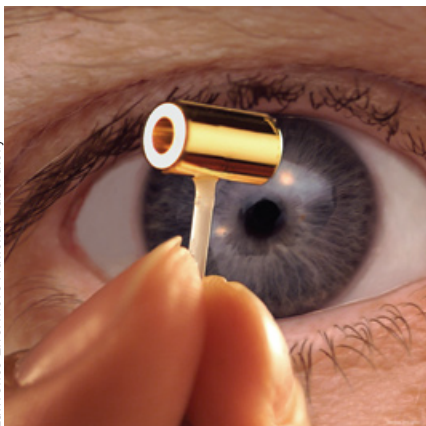
A NIF hohlraum. The hohlraum cylinder, which contains the NIF fusion fuel capsule, is just a few millimeters wide, about the size of a pencil eraser, with beam entrance holes at either end. The fuel capsule is the size of a small pea.
