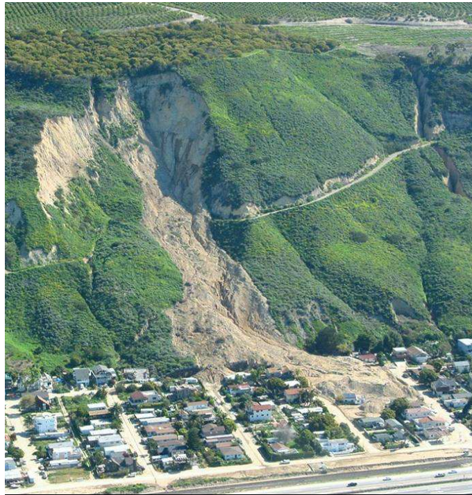
Figure 4.1. Site of the La Conchita, California landslide of January, 2005. This landslide was caused by massive rainstorms which soaked Southern California that winter (from Godt & Reid, 2005).
