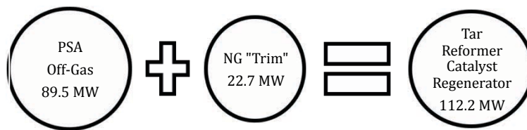
Figure 5.5 - Tar Reformer Catalyst Regenerator Flows
