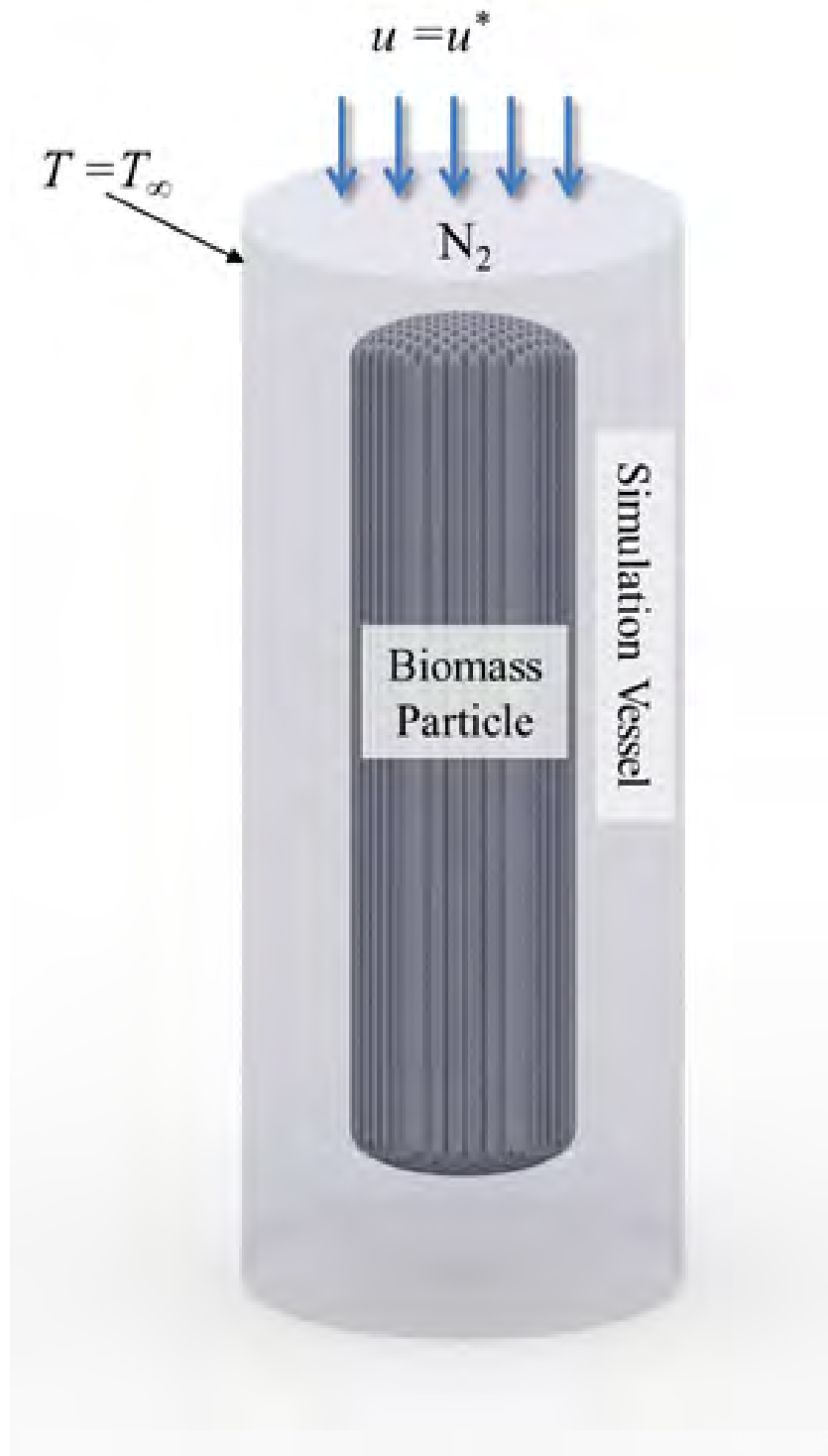
Figure 5.5: Schematic of the computational domain used for single particle simulations
