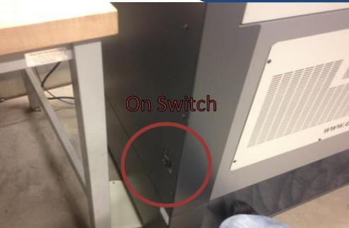
For vector cutting, begin by setting all line thickness' to hairline or 0.003". This will allow the Epilog machine to recognize a vector cutting operation. Turn on the Epilog Laser by switching the left panel power switch. Turn on the large white filter and compressor to the right of the Epilog as well. Load your materials into the laser by opening the top lid. Remove the focus triangle from the laser head and replace it upside down.
