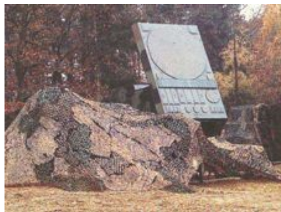
Figure 13. Phased-array radar for the Patriot missile system. (U.S. Defense Dept photo.)
