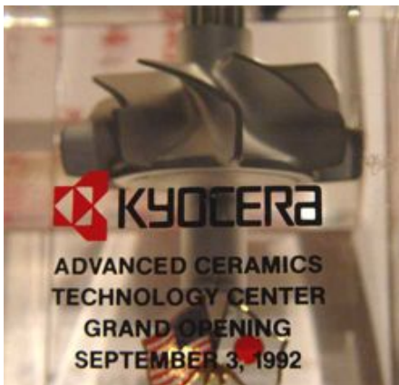
Figure 6. Souvenir from Kyocera plant opening with an imbedded silicon nitride— \text{Si}_3\text{N}_4 —turbo charger rotor. (D. W. Readey photo)
