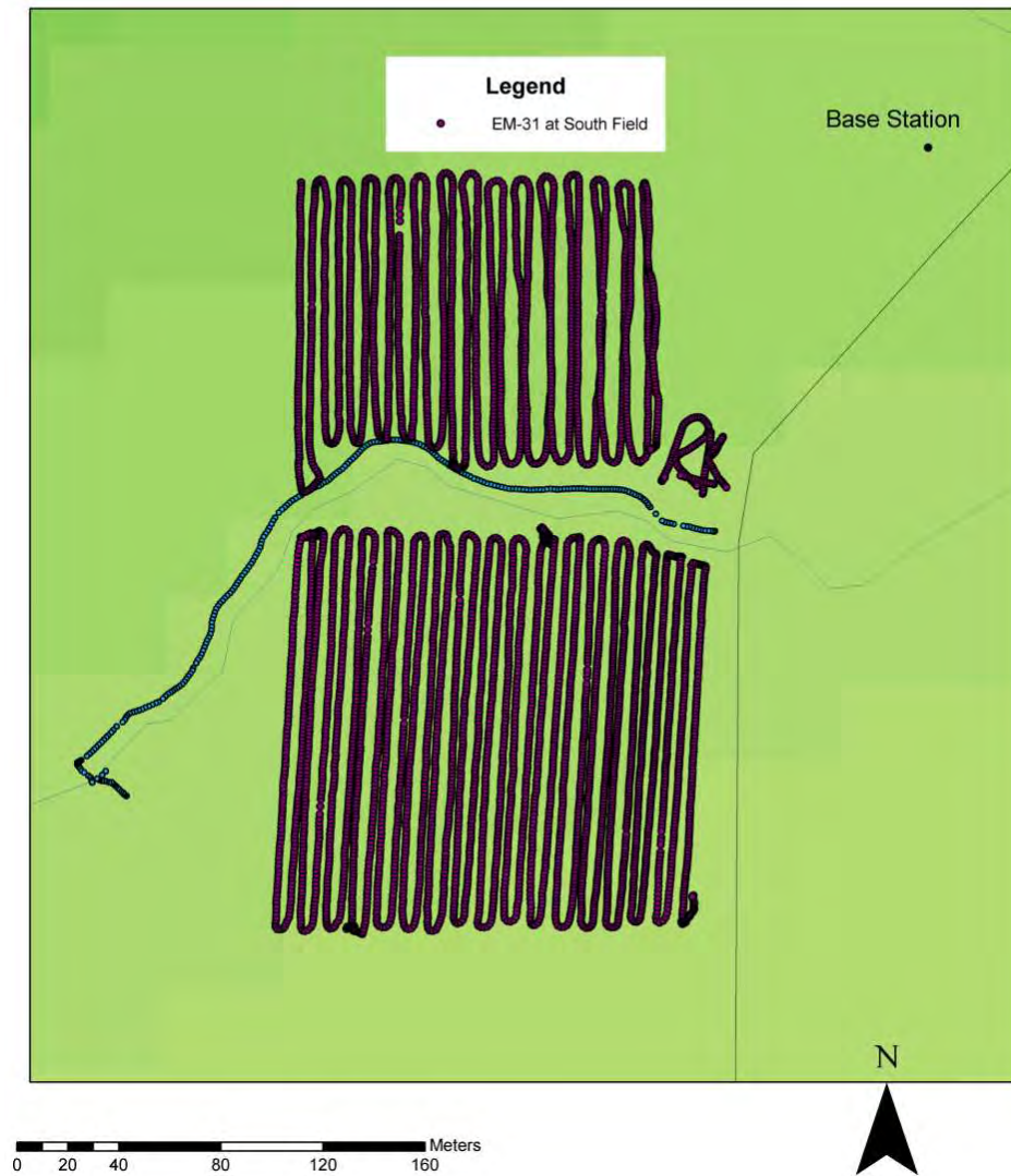
Figure 9.6.1: EM-31 Survey Line Locations and Geometry
