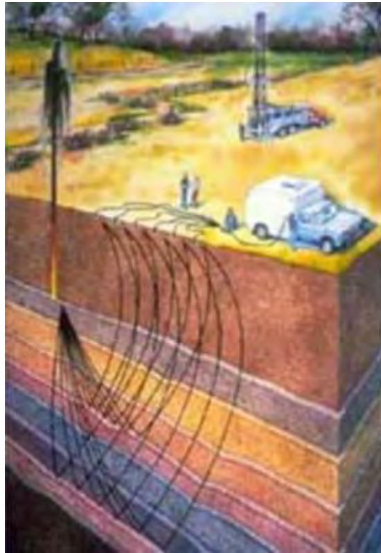
Figure 5.2.2: A schematic showing how seismic waves move through the Earth, reflect or refract, and then arrive at the surface to be recorded. This is the basic process for seismic surveying[10]
