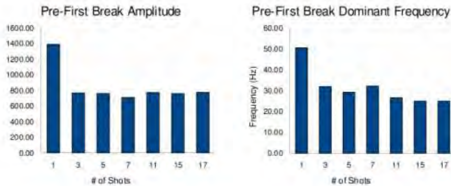
Figure 5.5.2: ProMAX statistics that were run for station 955 on the North line. The stacking was centered around shot gather 9 at this station. The pre-first break amplitude and frequency here are a measure of the ambient noise. As the statistics show, the ambient noise is attenuated rapidly by stacking these gathers together even though these gathers are really reshooting the same trace repeatedly. This kind of stacking is useful for attenuating incoherent noise.
