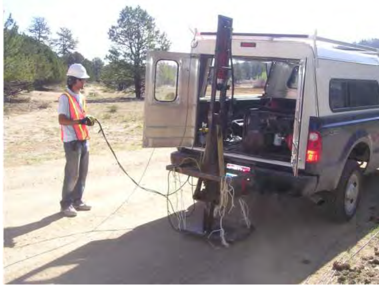
Figure 6.3.1: Weight drop system used in near surface seismic exploration
