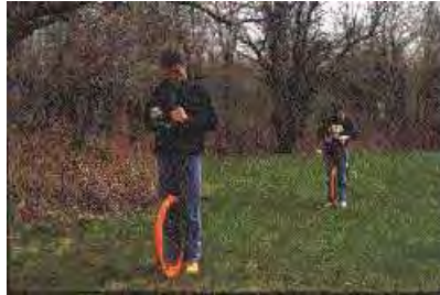
Figure 9.11.1: Alignment of transmitter and receiver loops ( http://www.geonics.com/em34.html )
