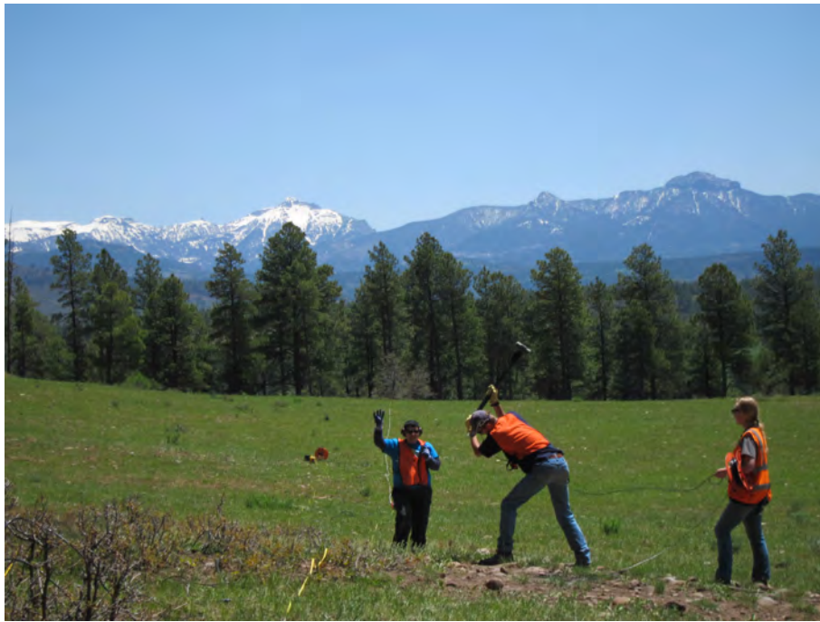
Figure 6.9: Photograph of hammer seismic survey being conducted over the east end of the student site. Pictured are crew members responsible for hammer swings and communicating between the recorder and swinger, as well as geophone and trigger cables.
