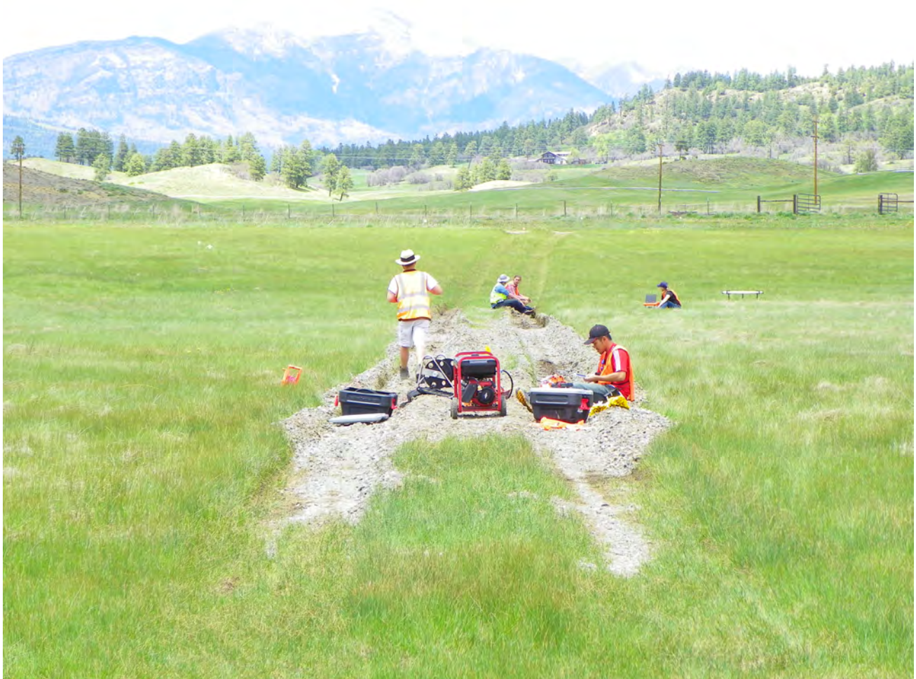
Figure 11.5: Photo of a TEM57 survey in progress on the Student Site. This was taken on May 23rd at Loop C, near the West end of the line. The transmitter controller and the generator power supply is in the center foreground, and the ProTEM and receiver loop are visible further back on the left. The transmitter loop extends almost to the fence in the background, about 50m beyond the receiver. Photo courtesy of Dawn Umpleby.
