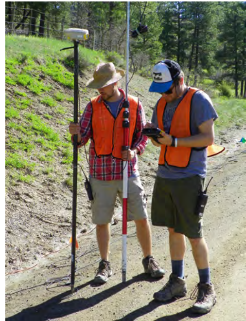
Figure 3.4: Student surveyors using the roving DGPS and antenna on the mainline.
