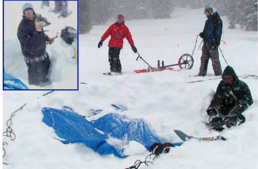
In the pit covered with blue tarp, Doug (shown in the inset) acquires data as Marc and Dustin pull the GPR antenna sled over a grid of buried objects. Jordan, in his usual position, performs as middle management, passing along commands.
