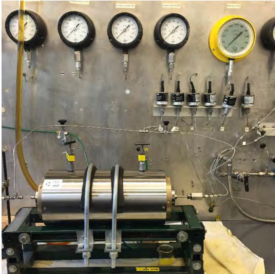
**Figure 21: Linear core holder unit**
