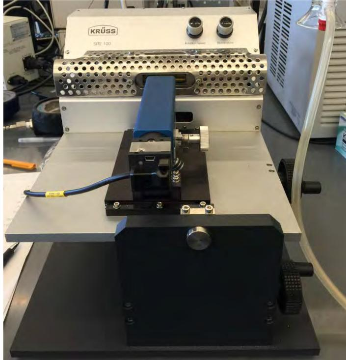
**Figure 16: KRÜSS Spinning Drop Tensiometer SITE100**
