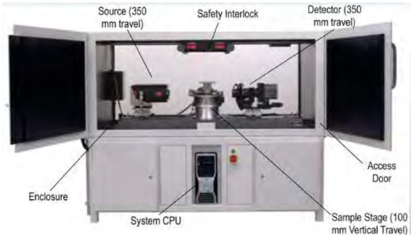
Figure 8: XRadia MicroXCT 400 (image adapted from catalog)
