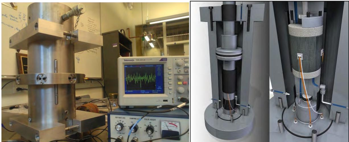
**Figure 30: Coupled Pore Pressure Penetration Apparatus (Triaxial Assembly)**
