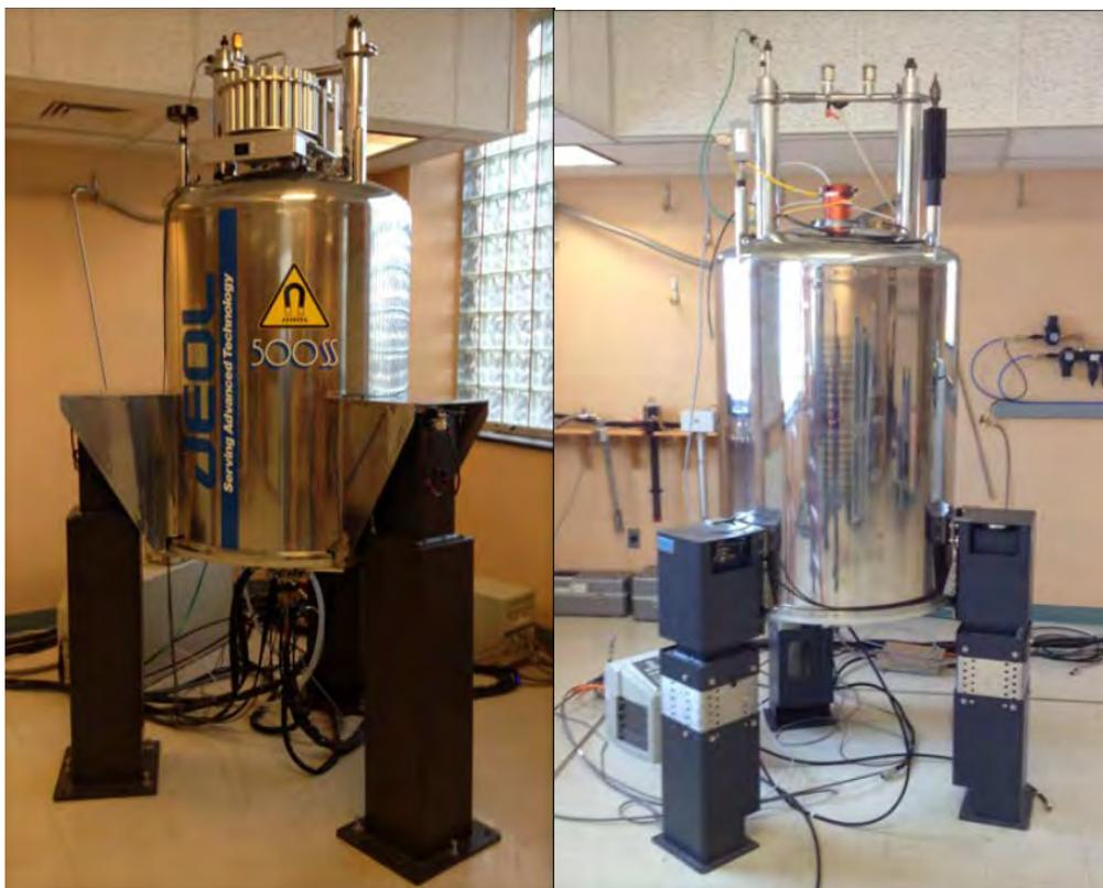
**Figure 47: 500MHz liquid-state (left image-adapted from CSM website) and 400 MHz solid-state NMR (right image-adapted from CSM website)**
