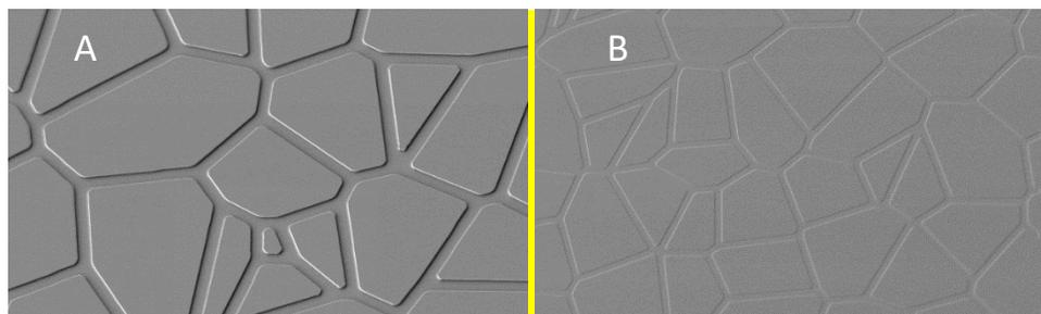
**Figure 10: Pore networks on nPMA. A – 300 nm channels; B – 30 nm channels**
