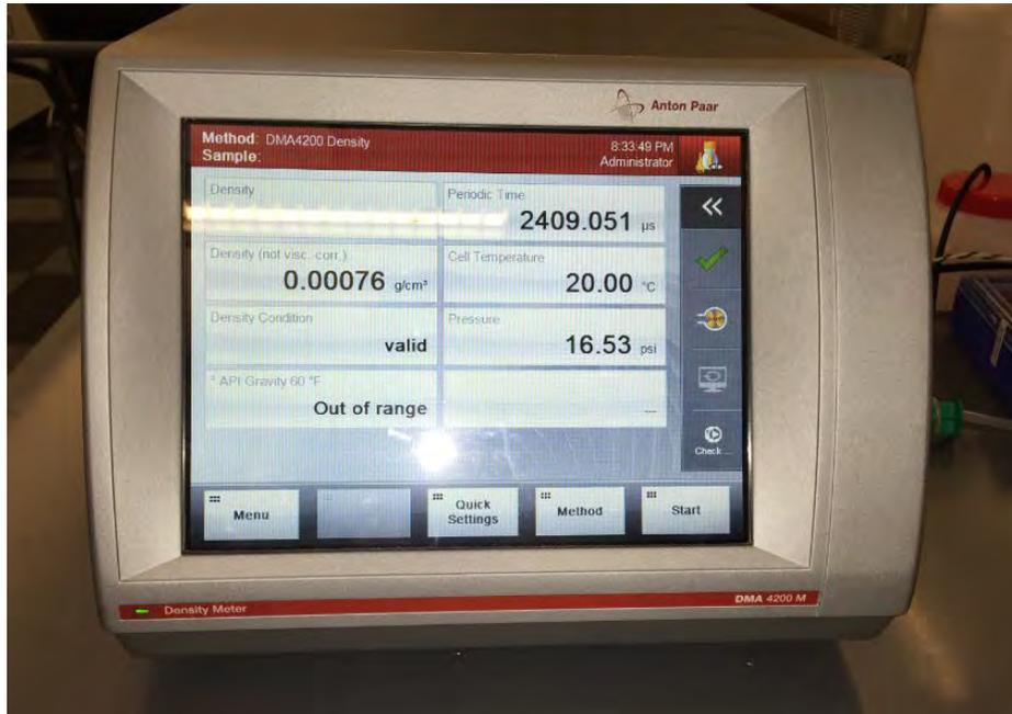
Figure 15: Anton Paar DMA 4200 M Densitometer
