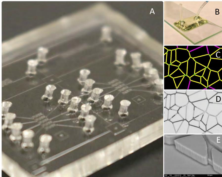
**Figure 9: A –  $\mu$ PMA “chips” being prepared on a master substrate; B – A fully assembled  $\mu$ PMA; C – A section of pore network etched onto  $\mu$ PMA; D – Water flooding pattern in the same section; E – SEM image of channels in a  $\mu$ PMA**
