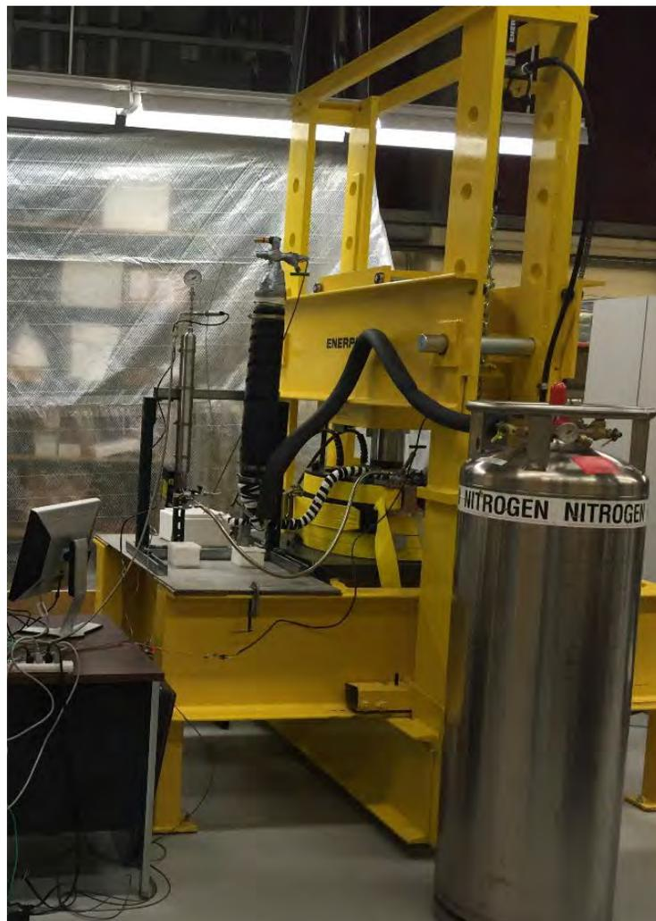
**Figure 33: Hydraulic fracturing system with tri-axial stress loading**
