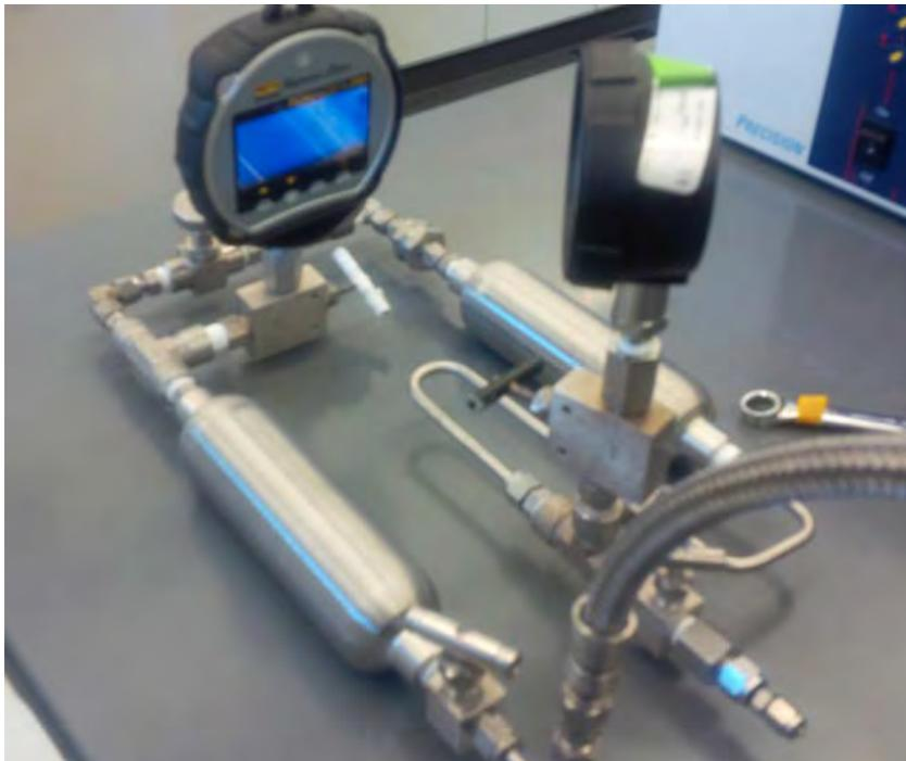
**Figure 3: Gas Adsorption System**
