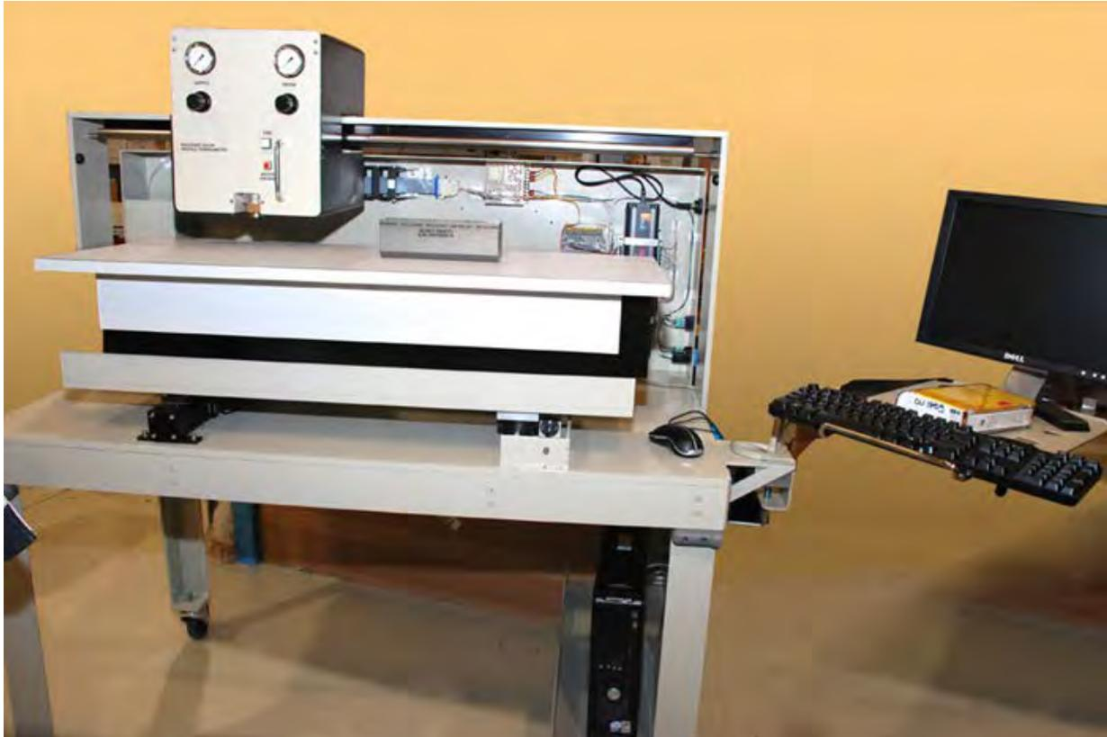
Figure 2: Core Lab PDPK™-400, Pressure-Decay Profile Permeameter (image adapted from catalog)
