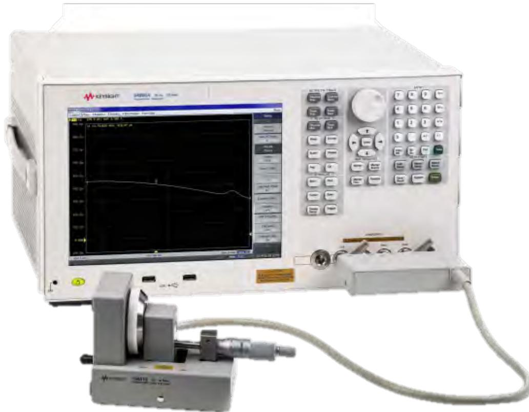
**Figure 24: Impedance Analyzer (Keysight manual)**
