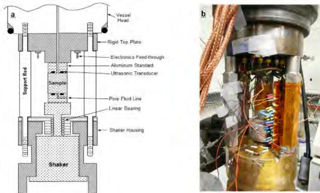
**Figure 6: (a) Schematic of the low frequency measurement assembly. For seismic frequencies, strains are measured on both the sample and aluminum standard. Ultrasonic transducers permit wave propagation measurement near 1 MHz. Fluid lines permit control and exchange of pore fluids independent of confining pressure, (b) Photograph of completed measurement assembly**
