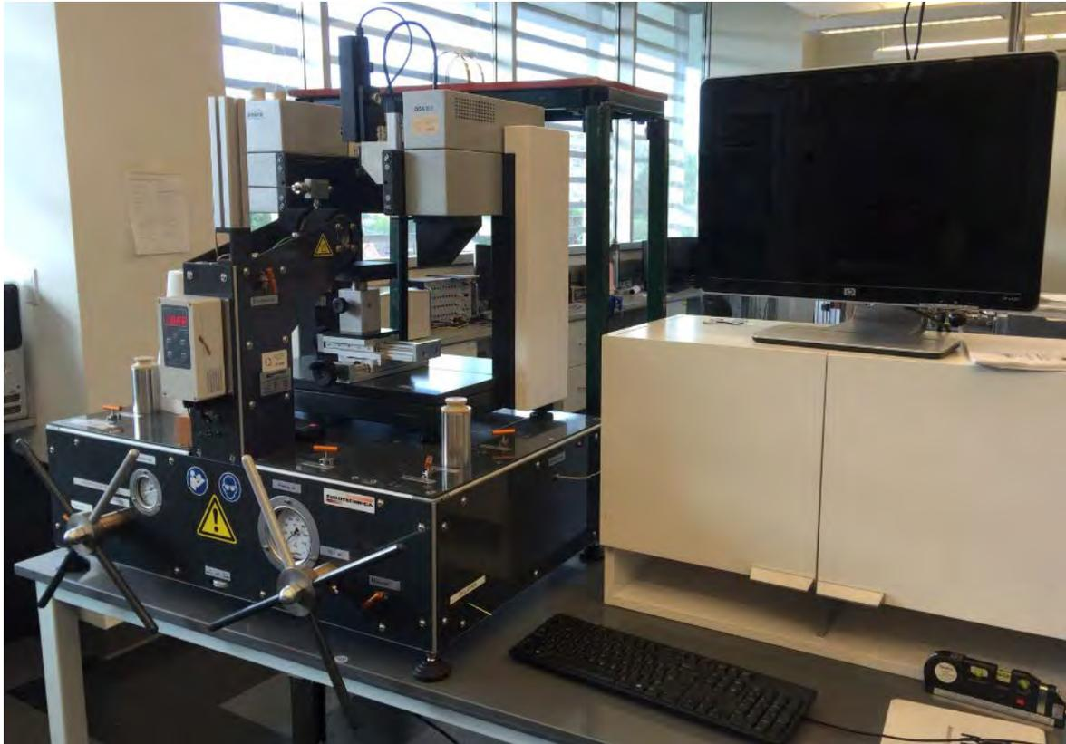
**Figure 22: KRÜSS Drop Shape Analyzer DSA100**
