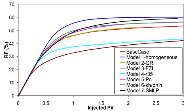
Recovery Factor versus Injected Pore Volume
