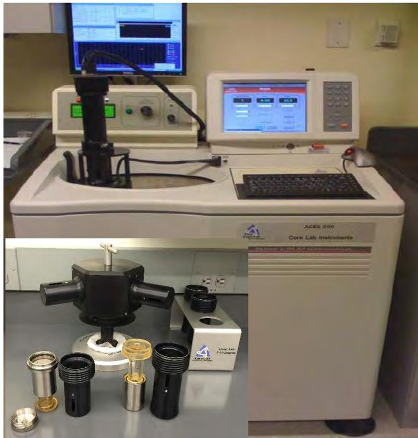
Figure 18: Core Lab ACES-200 Automated Centrifuge System
