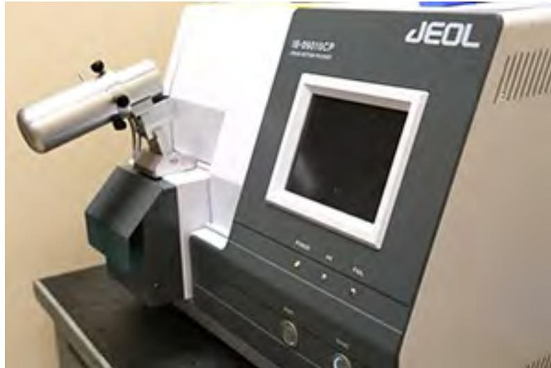
**Figure 43: The JEOL cross-section polisher**
