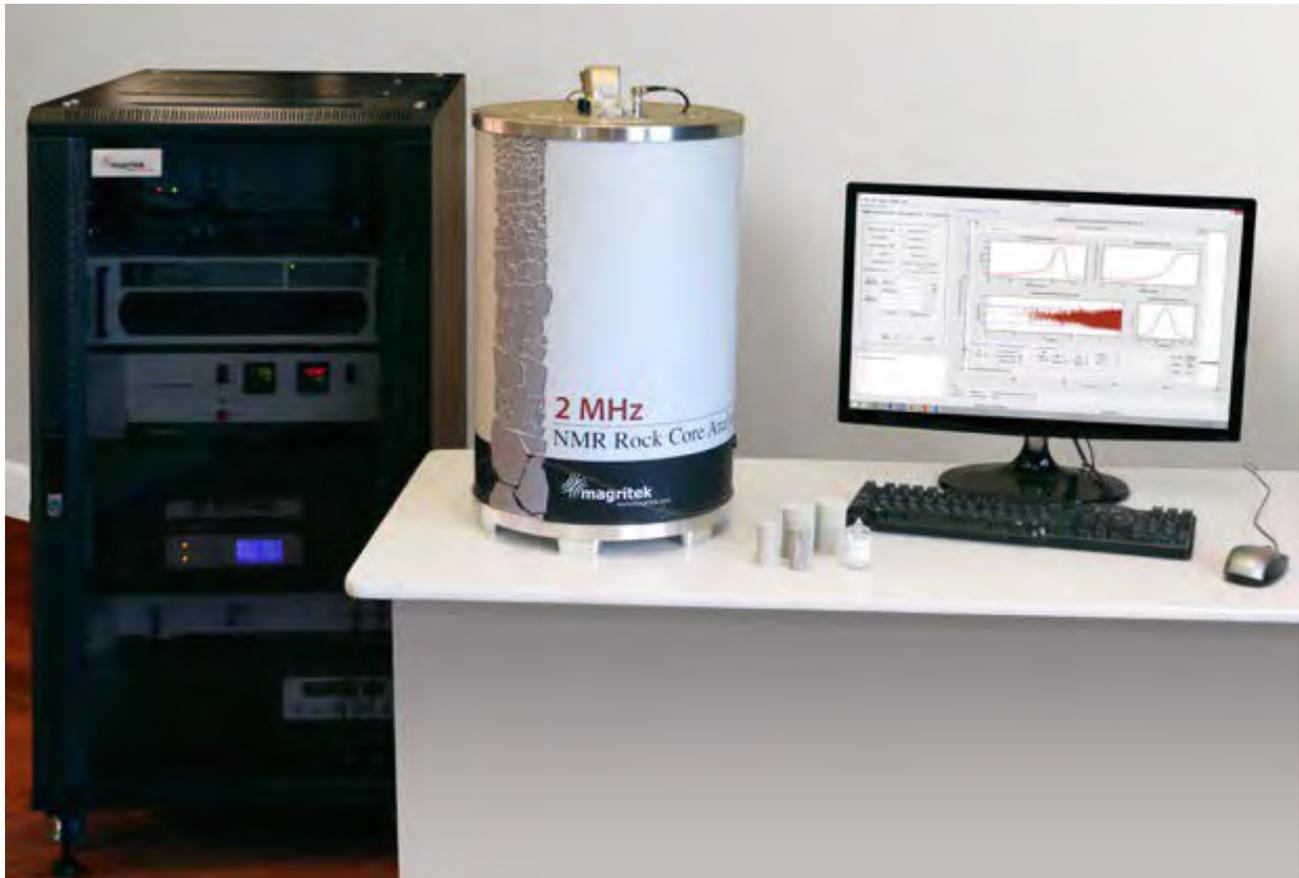
Figure 28: 2-MHz Magritek NMR laboratory setup for core analysis (Magritek website)
