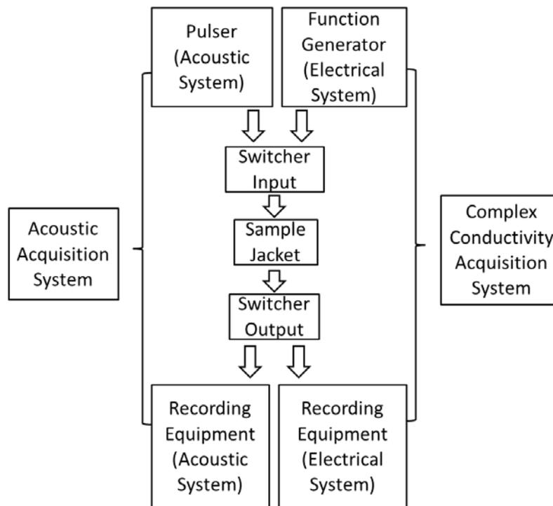
**Figure 26: Schematic of anisotropic acoustic – electrical joint measurement system**
