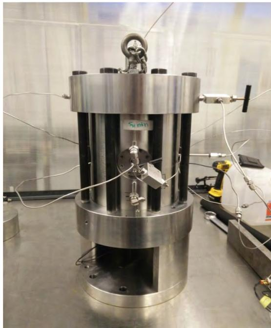
**Figure 29: Coupled True Triaxial Core Measurement Assembly**
