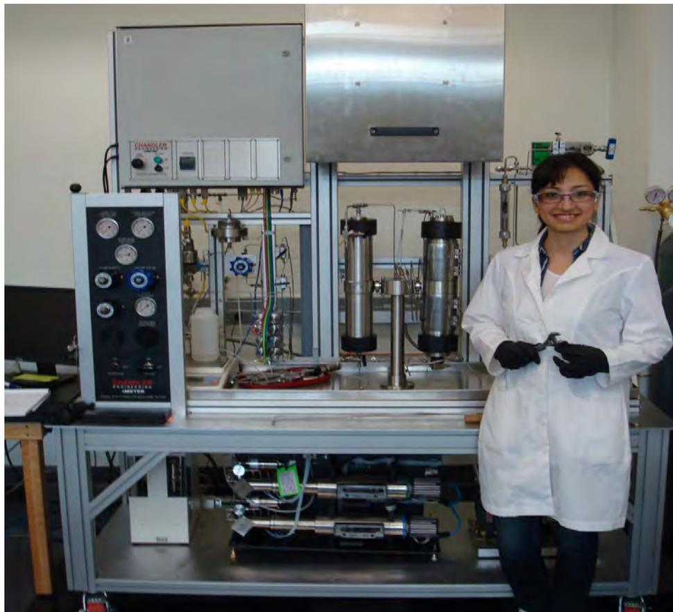
**Figure 20: Chandler Formation Response Tester (FRT) 6100 Core Flooding System**
