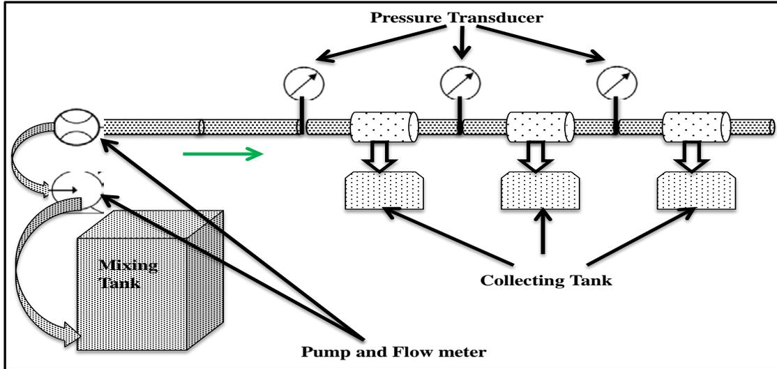
**Figure 34: Schematic of proppant transport in horizontal wellbore experimental setup**
