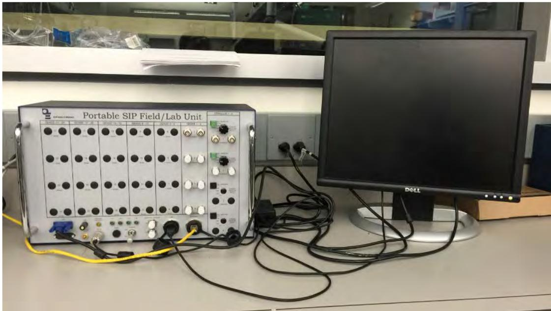
**Figure 23: Resistivity Measuring Instrument**
