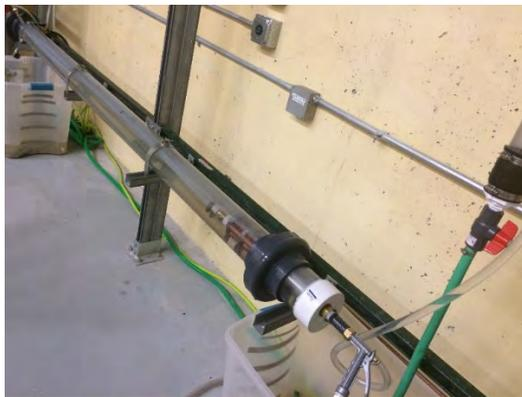
**Figure 38: Casing with Mandrel inserted**
