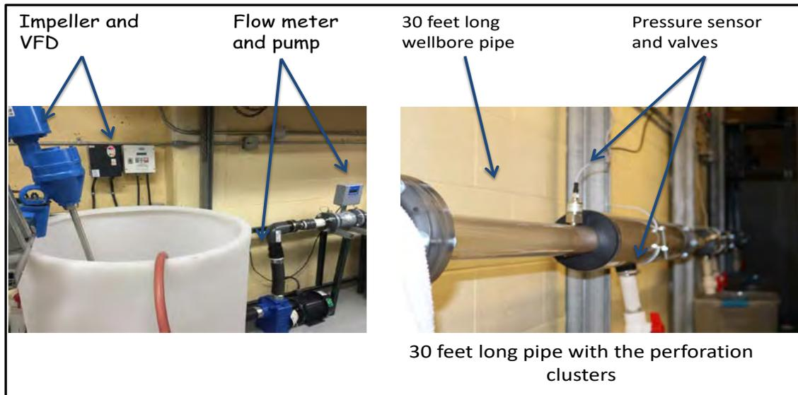
**Figure 35: Images of proppant transport in horizontal wellbore experimental setup**
