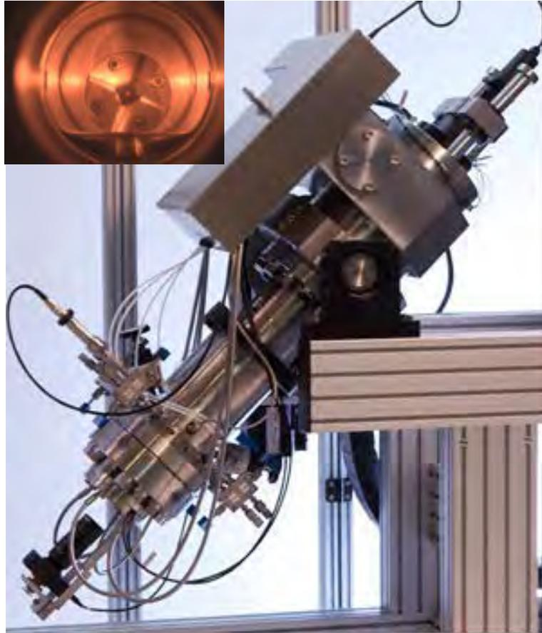
**Figure 13: PVT cell at 45 ° from horizontal to capture condensate accumulation, and a view of the cell interior on the top left corner (modified from Core Lab catalog)**
