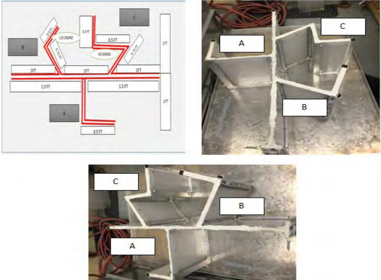
**Figure 36: Schematic and images of experimental setup used to study proppant transport in a complex fracture system**
