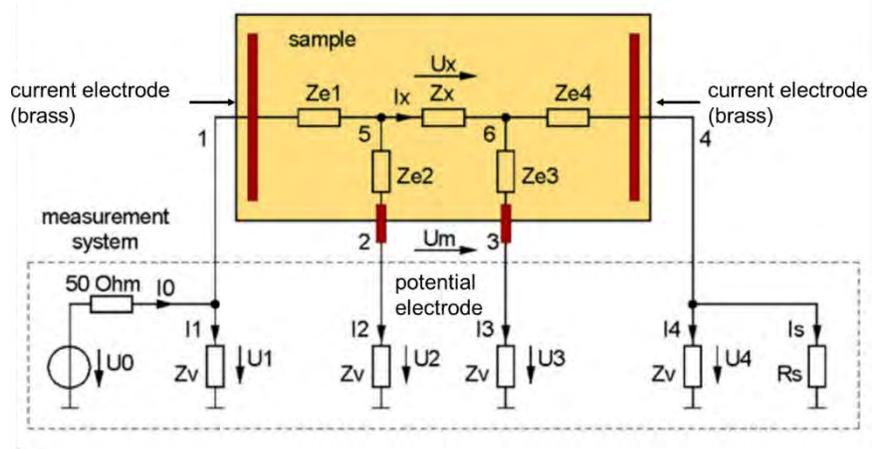
**Figure 27: Electrode array and circuit simplified diagram of SIP system. 1 and 4 represent current electrodes, 2 and 3 represent potential electrodes. (Adapted from Zimmermann et al., 2008)**
