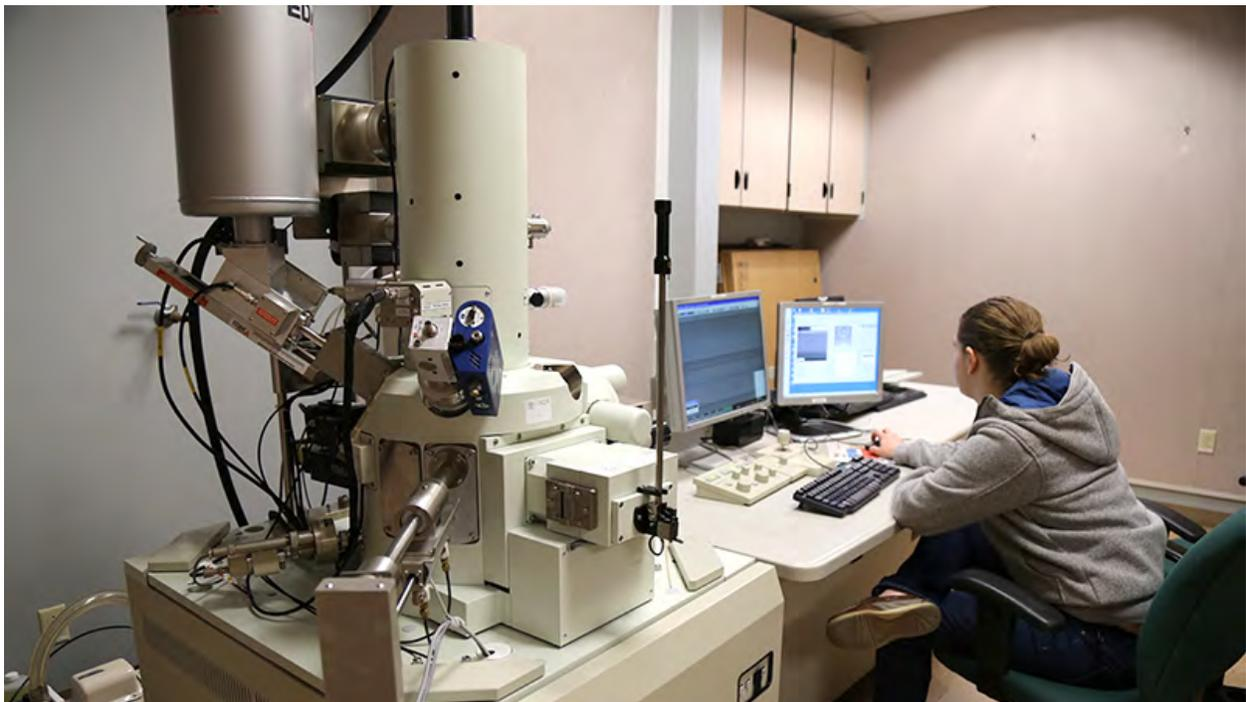
**Figure 42: Field Emission Scanning Electron Microscope (FE-SEM)**
