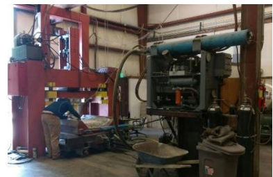
Fig. 3: Large-scale linear cutting test setup.
